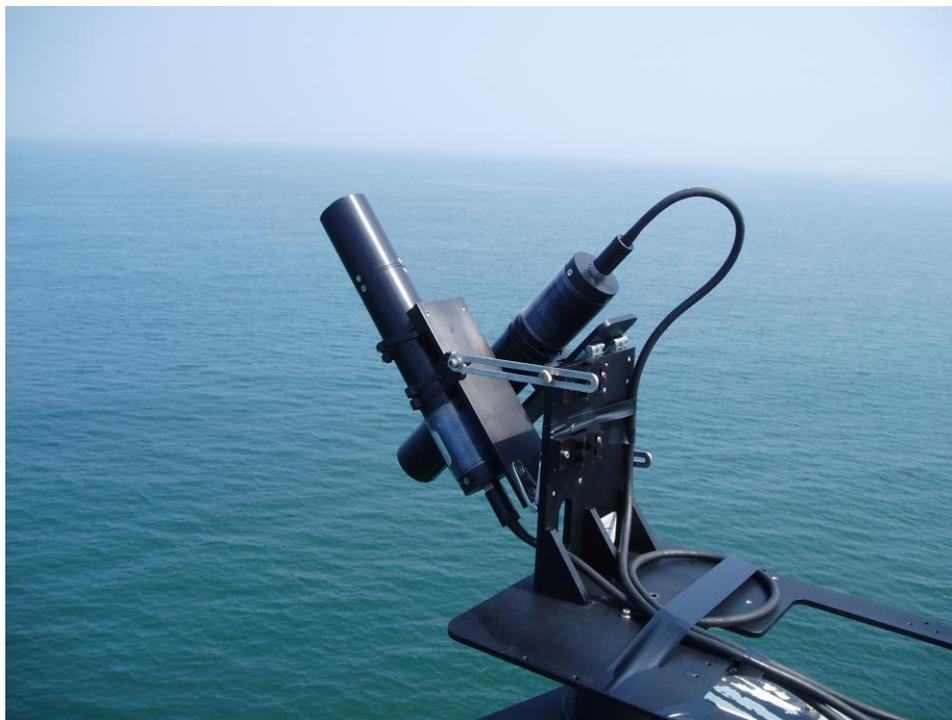
**Figure B.3:** Photo of commercial ocean color radiometers (photo courtesy of Satlantic HyperSAS).
